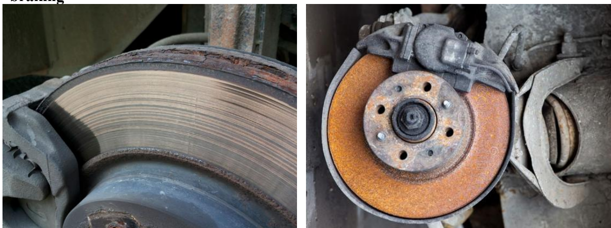
c) Noise in improper eating d) Wear out brake discs.
