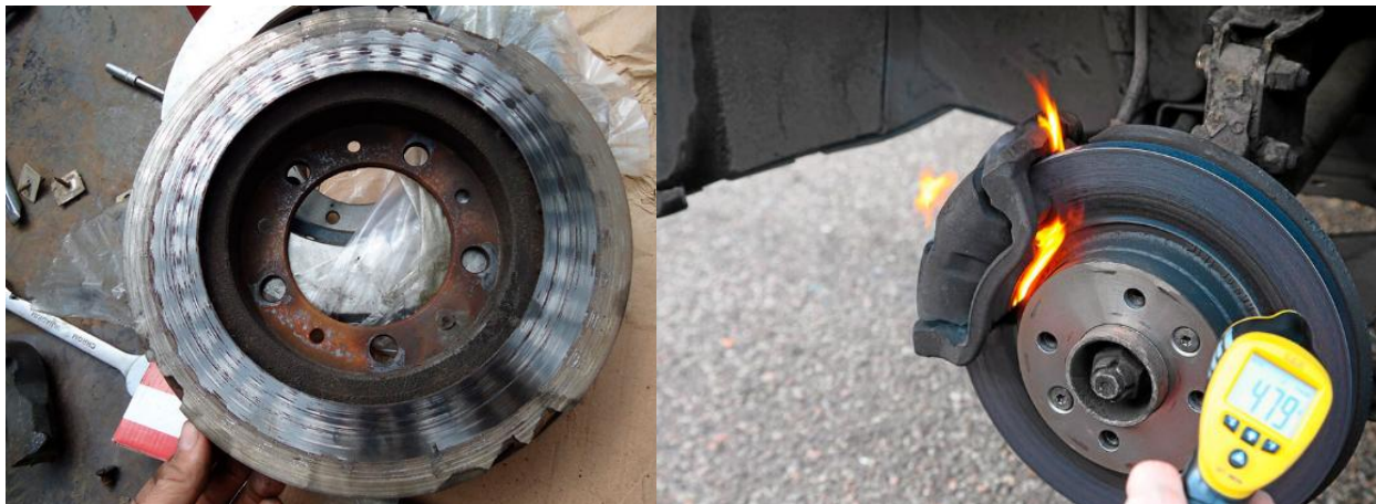
Picture-3. a) vibration generation when braking b) overheating the brakes very quickly
