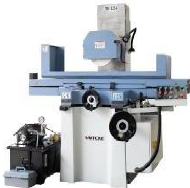
Figure 1. MY1224 grinding machine for mechanical processing of welded flat-surface parts
