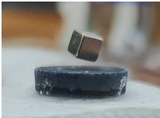
Figure 1. The Meissner effect in a YBCO sample.
