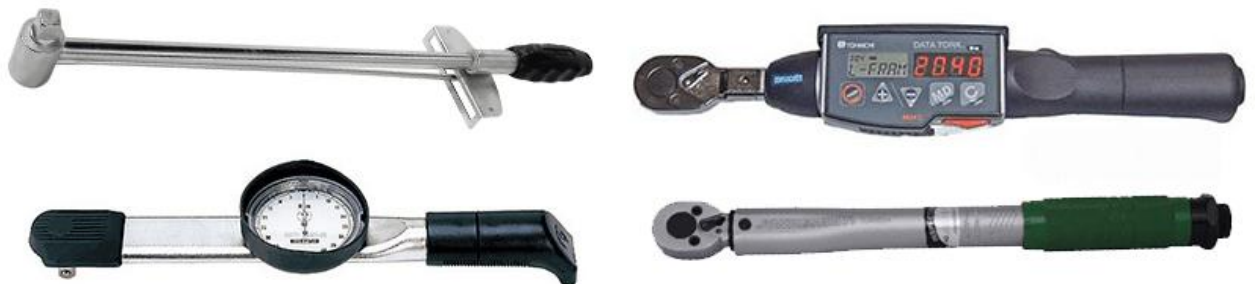
Figure 2. Dynamometric keys and their types
