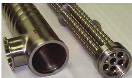
Fig. 2. Configurations of profiled-tube heat exchangers manufactured by HRS Group (Spain).
