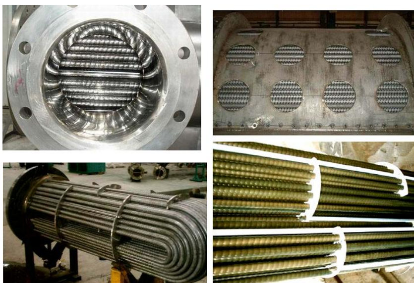
Fig. 2. Configurations of profiled-tube heat exchangers manufactured by HRS Group (Spain).
