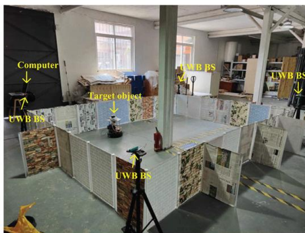
(a) Experimental environment for UWB-based UGV localization.
