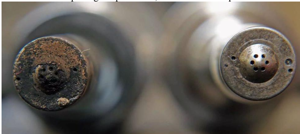
Figure 4. The condition of the injector hole.
