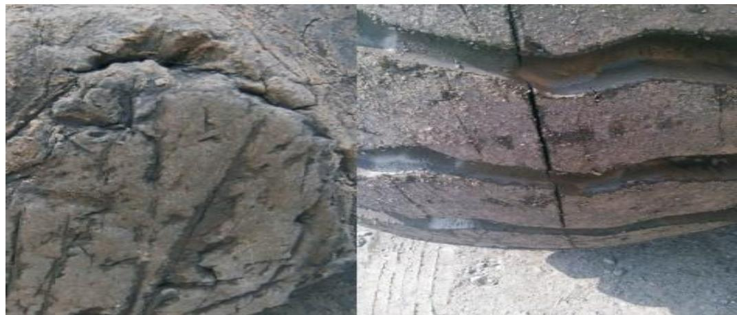
3. **Internal cord breakage** – the loss of strength of a metal or textile cord as a result of prolonged heat exposure.
