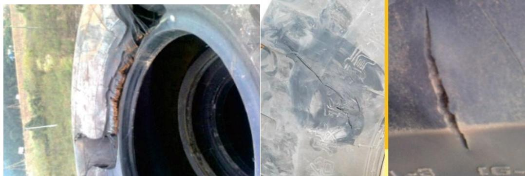
2. **Tread separation** occurs as a result of the tire's inner layers overheating.
