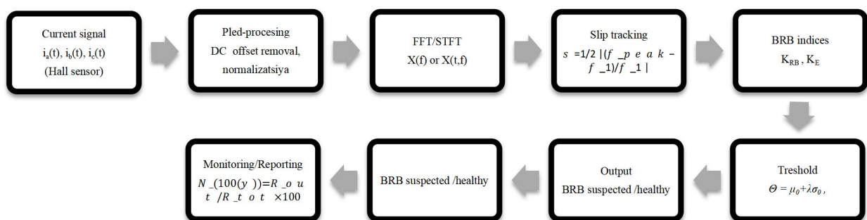
Figure 5 (algorithm): Block diagram based on MCSA for early detection of BRB.
