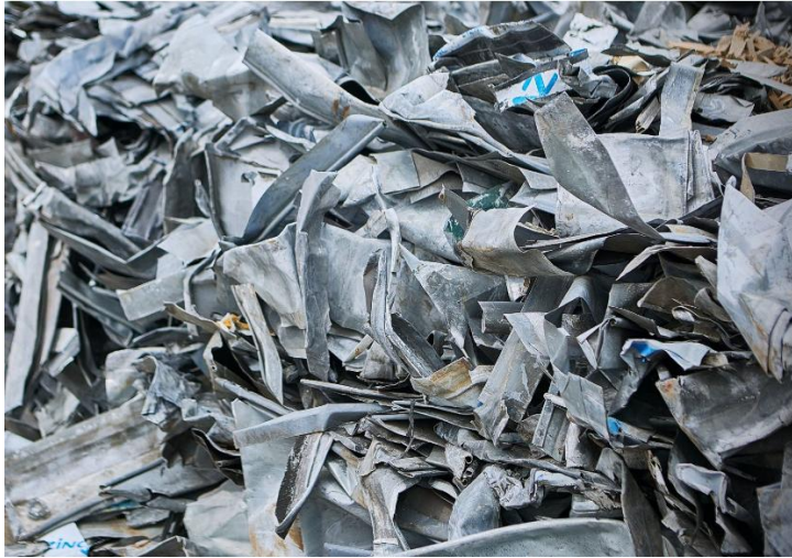
Fig. 2. Fragments of aged zinc sheet waste
