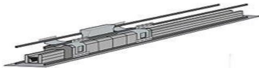
Figure 4. View of the EMALS asynchronous motor.
