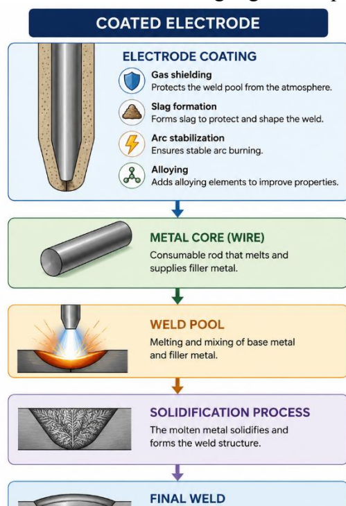
Figure 3. Schematic Representation of Weld Formation Using a Coated Electrode
