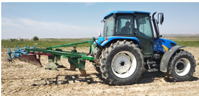
Fig.4. General view of the combined machine in the unit with the tractor T 100 A (side view)
